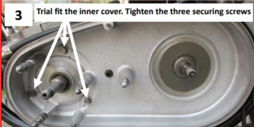
Correctly shimming the inner case means the primary cases do not distort when the single fixing nut is tightened
